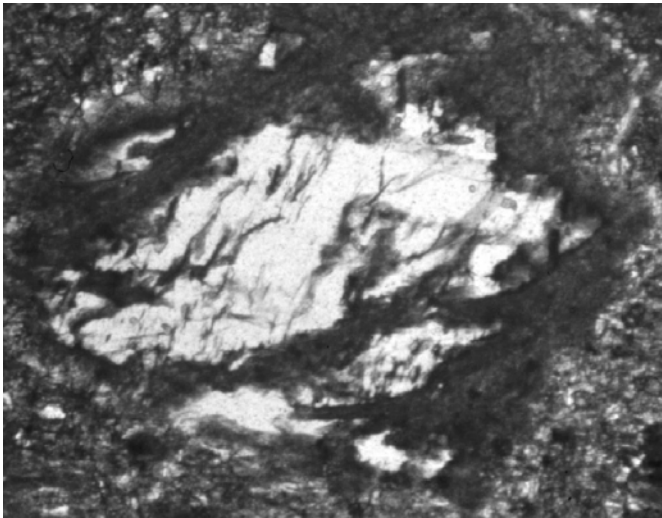
Fig. 3.3-11: Photomicrograph in plane polarised light showing a partially altered clinopyroxene crystal from the A3 section of Rovic 124 eclogite (Roberts Victor, South Africa). The grain is approx. 1 mm in diameter.
