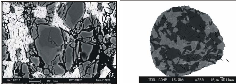
Fig. 3.4-18: Left: A recovered sample from 1400\text{ }^\circ\text{C} showing light \text{CaSiO}_3 perovskite surrounding darker garnet grains. Significant zoning of the garnet grains can be seen due to the incomplete reaction with \text{CaSiO}_3 . Right: A similar sample from 1600\text{ }^\circ\text{C} where zoning is no longer apparent (SEM-BSE images).
