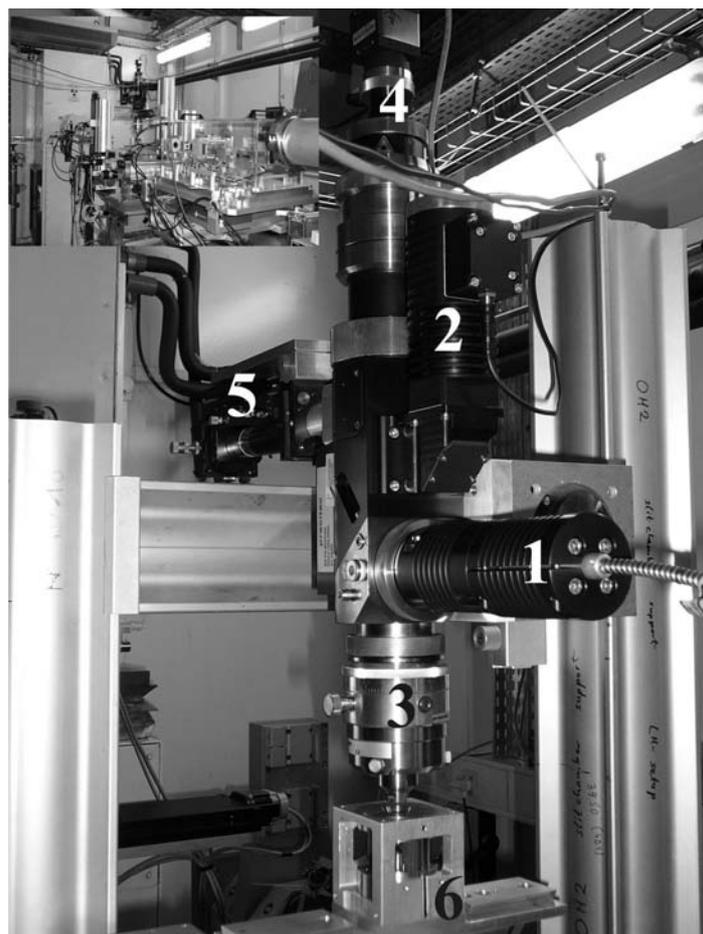
Fig. 3.10-1: The Universal laser-heating head (UniHead) mounted at ID18 beam line at ESRF (see inset) for nuclear inelastic scattering experiments in diamond anvil cells (1 – the connector for SPI100 fiber laser, 2 – the illumination unit, 3 – the lenses unit for focusing of the incoming laser light, 4 – the digital video camera, 5 – the module for spectroscopic measurements, 6 – the diamond anvil cell mounted inside the holder).
