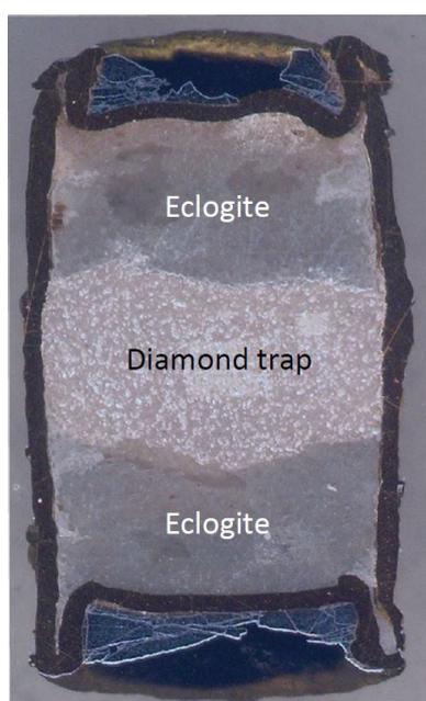
Fig. 3.2-19: A capsule with a diamond trap layer between eclogite recovered from a piston cylinder experiment at 4 GPa and 800 °C. The capsule width is approximately 5 mm.
