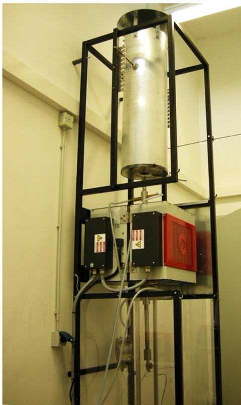
Fig. 3.8-15: A new apparatus for studying magma fragmentation in andesitic and basaltic systems. A TZM alloy autoclave is located inside the furnace (red). Both ends of the autoclave are water-cooled. At the top of the autoclave (above the furnace) is a ruptured disc that will fail at a pre-determined pressure. Material erupted from the autoclave is collected in the large tank at the top of the apparatus.
