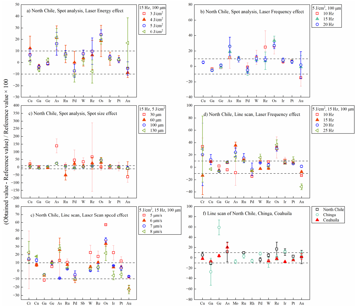
Fig. 3.8-4: Accuracy and precision of chemical analysis represented by the differences in mean composition and one standard deviation of elements with reported bulk compositions obtained by INAA. a.-e. The effects of laser energy, frequency, spot size and scan speed of spot analysis and line scan on the chemical analysis of North Chile were tested sequentially. f. The accuracy and precision of chemical analysis in North Chile, Chinga, Coahuila were determined using the line scan of LA-ICP-MS with 100 \mu\text{m} width, 6 \mu\text{m/s} scan speed, 5 \text{J/cm}^2 energy fluence, 20 Hz frequency.
