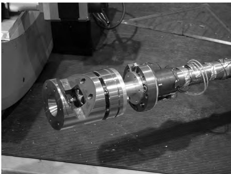
Fig. 3.10-5: Diamond anvil cell mounted on the top of the cryostat cold finger for a HP experiment at FRM II using Stress-Spec diffractometer.
